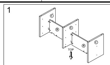
Attach the two End Base (C) and Center Base (E) to Modesty Panel (B) by using Cam Lock (C1) and Klix Cam (C2).
