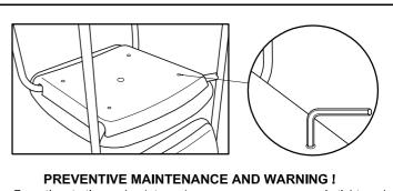
• From time to time, check to make sure screws are securely tightened. Delta Holes on PP shell are for convenient checking.
