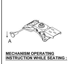
(A) SEAT HEIGHT ADJUSTMENT: Pull lever up and downward. Release lever when desired position is reached.
