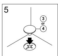
Attach Housing Cap (3 or 4) to all Klix Cam(2) by pushing neck thought center of cam.
