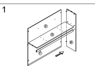
Attach the Fixed Shelf (D) and Back Panel (E) to Side Panel (B) by using Cam Lock (1) and Klix Cam (2). Attach the Center Rail (F) and Side Panel (B) by using assembled hardware-Wood Dowel.
