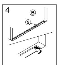
Peel Double Sided Foam Tape (5) and stick it on bottom of Side Panel (B).
