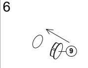
Insert the Hole Plug (9) to all drill hole of the Side Panel (B) and Center Vertical Panel (C).
