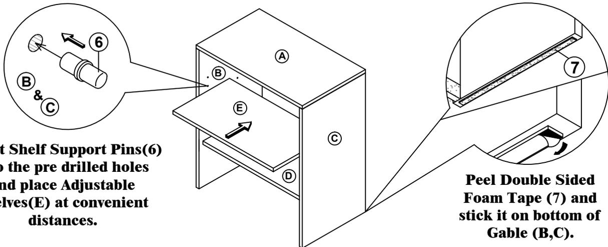
**Insert Shelf Support Pins(6) into the pre drilled holes and place Adjustable Shelves(E) at convenient distances.**
