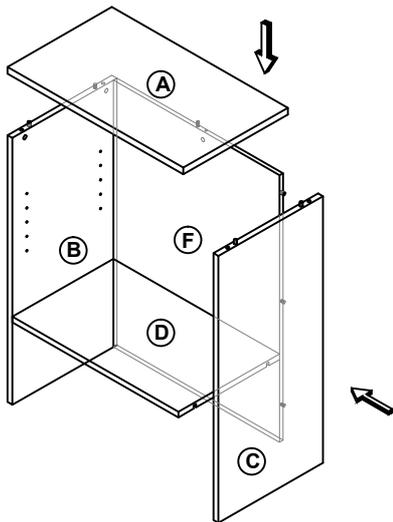
**Attach Right Gable(C) to Fixed Shelf(D) by using System 6 Fitting(5) . Attach Top Panel(A) to Left Gable(B) and Right Gable(C) by using Cam Lock(1) and Klix Cam(2).**
