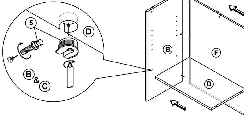
**Attach Fixed Shelf(D) to Left Gable(B) by using System 6 Fitting(5) and Back Panel(F) by using Cam Lock(1) and Klix Cam(2).**
