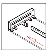
Screw the desk riser to the table top with bolts M6 X 16mm (part 3). Then, slide in the beam.
