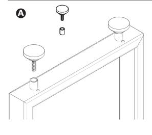
Place plastic spacer over threaded insert on PLTLP-HS unit.
